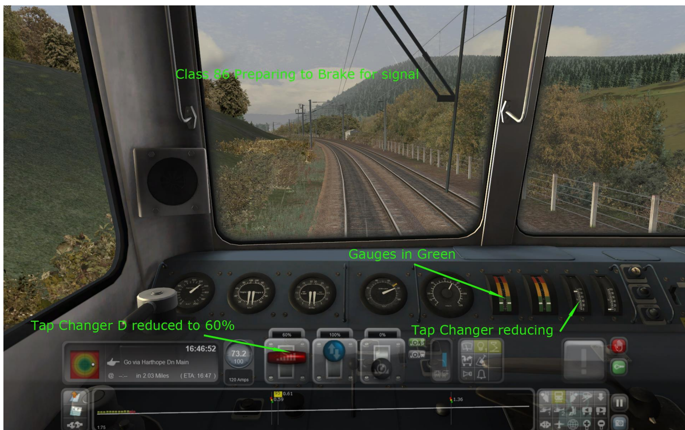
Position of the gauges and tap changer as we start to slow down and prepare for braking.
