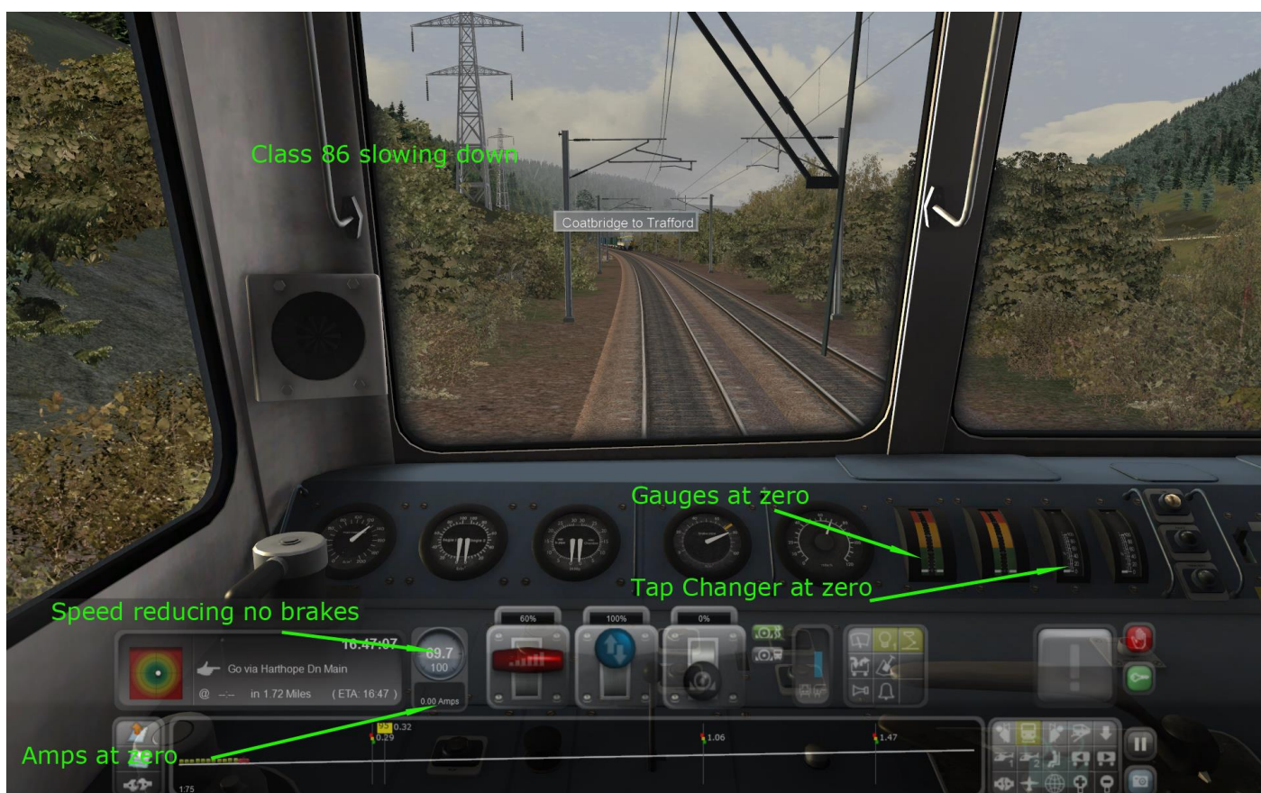
Further speed reduction. Using "D" reduced amps to zero i.e. no power
