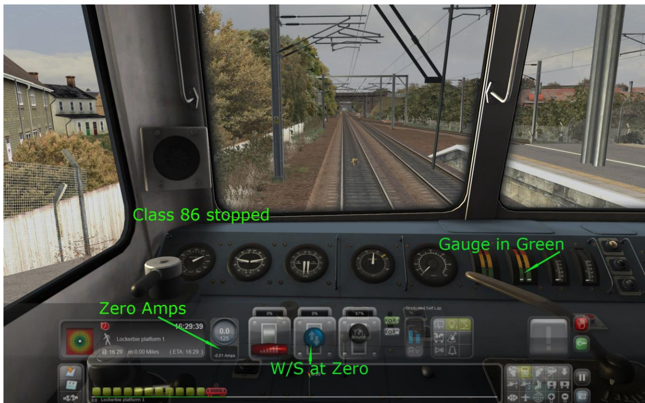
This is the Class 86 stopped at a station. Note the positions of the controls
